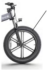
Seat the axial stem properly within the receptacles at the tips of the fork.
